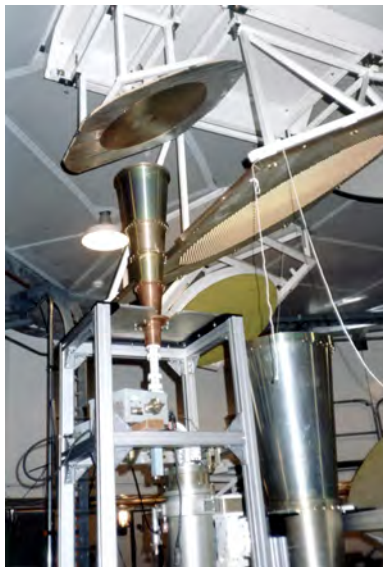
Fig. 7-47. DSS-13 S/X-band feed-system geometry.
