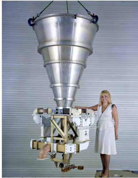
Fig. 6-2. Photograph of the R&D common-aperture feed horn.
