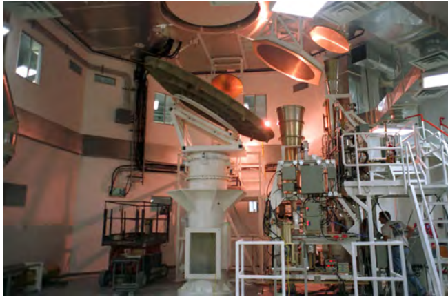
Fig. 8-8. The S-/X-band feed system at DSS-24.
