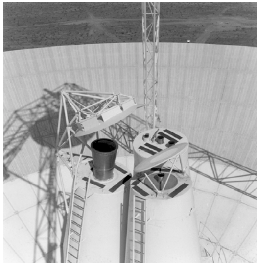
Fig. 5-19. Reflex–dichroic feed on the 64-m antenna.
